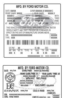
Image: state **WARNING:** Exceeding the Safety Compliance Certification Label vehicle weight rating limits could result in substandard vehicle handling or performance, engine, transmission and/or structural damage, serious damage to the vehicle, loss of control and personal injury.
